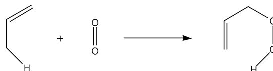
Figure 4. Allyl hydroperoxide formation by an ene -reaction between a singlet oxygen molecule and a C–C double bond system, which contains at least one allylic hydrogen atom.
